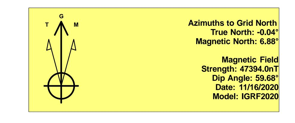
To convert a Magnetic Direction to a Grid Direction, Add 6.88° To convert a Magnetic Direction to a True Direction, Add 6.92° East To convert a True Direction to a Grid Direction, Subtract 0.04°
