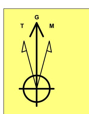
**Azimuths to Grid North** True North: -0.04° Magnetic North: 6.87°
