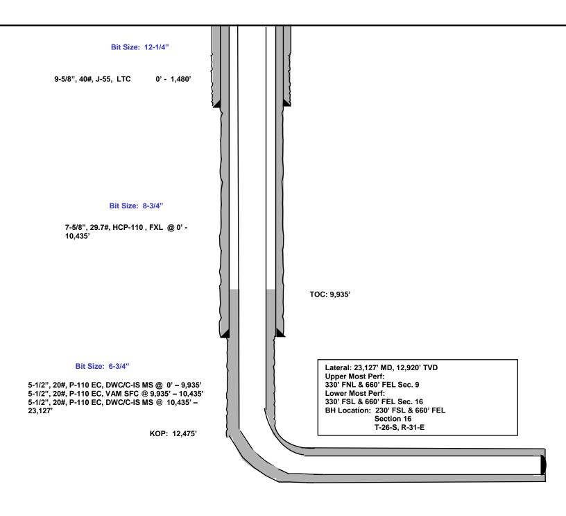
554' FSL 1,313' FEL Section 4 T-26-S, R-31-E Proposed Wellbore Design B KB: 3,311' GL: 3,286'
