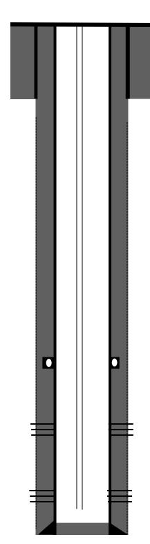
9-5/8" L-80, 47# casing @ 163'. Cemented with 136 Class B. Circulated to surface. Hole size 12-1/4"
