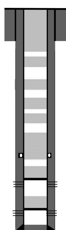
9-5/8" L-80, 47# casing @ 163'. Cemented with 136 Class B. Circulated to surface. Hole size 12-1/4"
