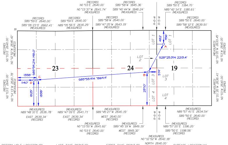
BOTTOM HOLE LOCATION (D) 1825' FSL 1140' FWL SECTION 23, T31N, R6W LAT 36.8828740°N LONG -107.4366811°W DATUM: NAD1927 585°59.2'W 198.0'
