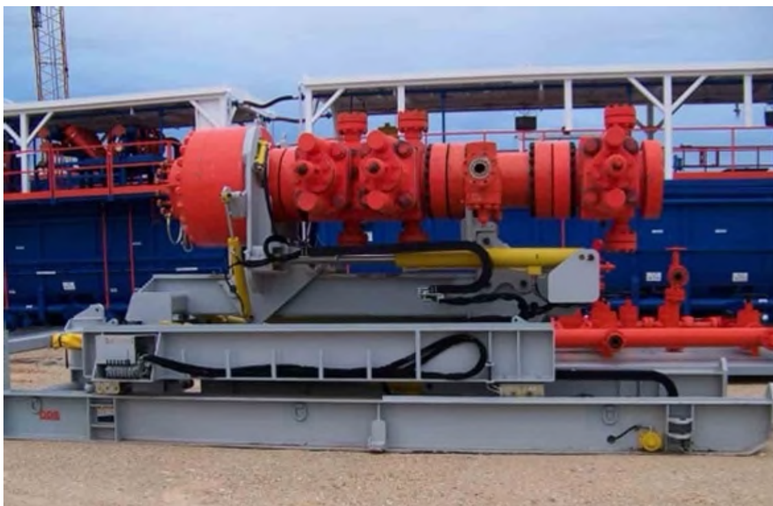
Figure 4. BOP handling system
