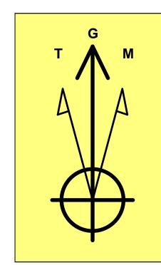
**Azimuths to Grid North** True North: -0.44° Magnetic North: 5.78°
