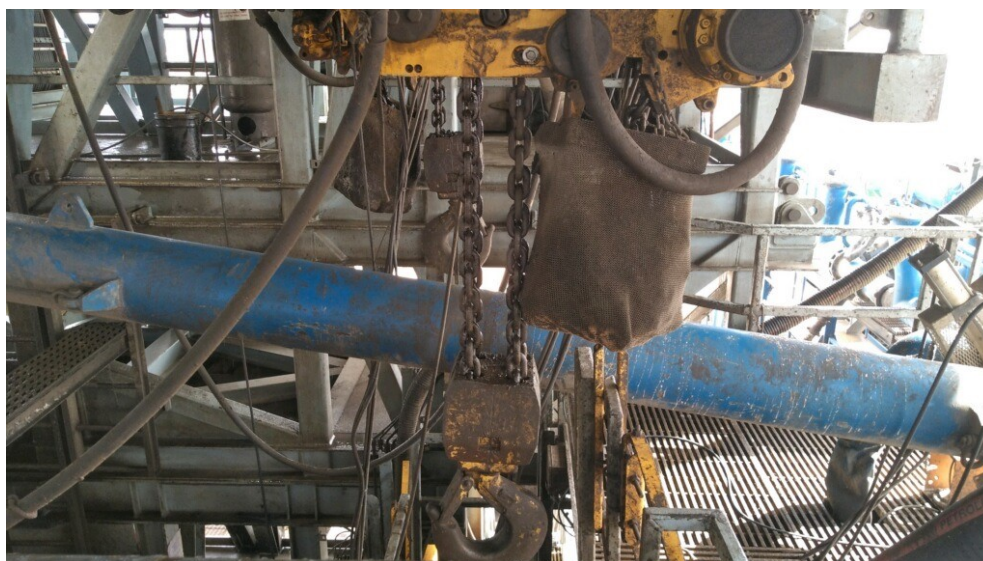
Figure 2: BOP Winch System
