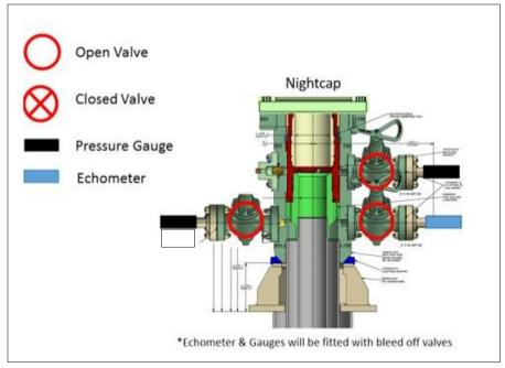
Wellhead diagram during skidding operations
