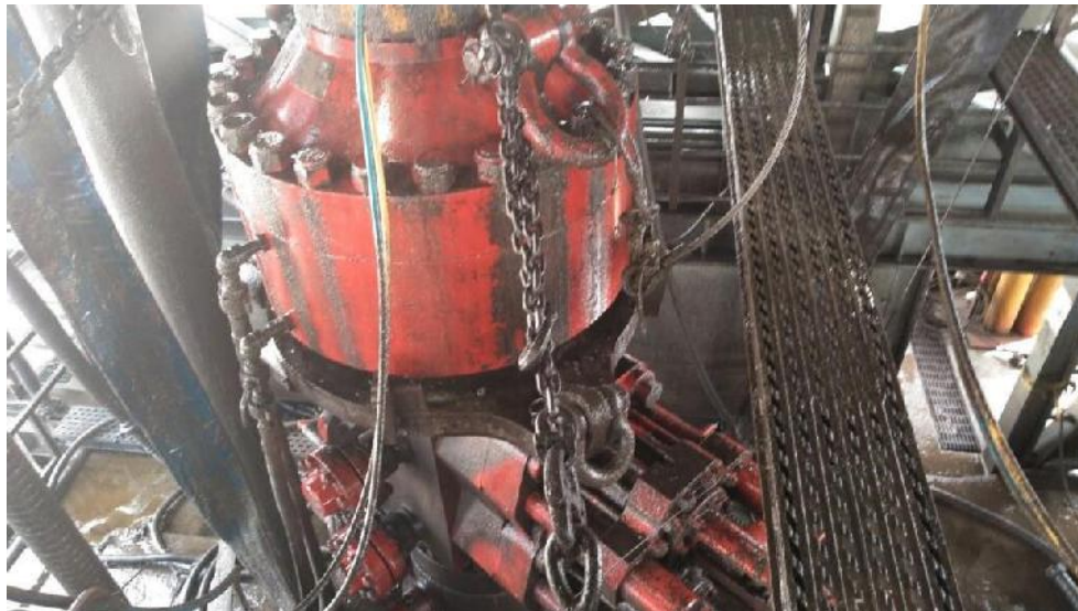
Figure 1: Winch System attached to BOP Stack
