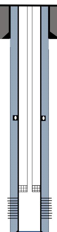
**Surface Casing:** 8-5/8", 24# J-55 casing set @ 244' **Cement Job**: 170 sks, Class B cement. Circulated 8 bbls to
