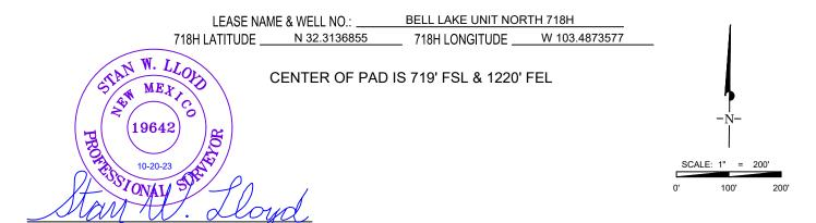
ALL BEARINGS, DISTANCES, AND COORDINATE VALUES CONTAINED HEREON ARE GRID BASED UPON THE NEW MEXICO COORDINATE SYSTEM OF 1983, EAST ZONE, U.S. SURVEY FEET. ELEVATIONS USED ARE NAVD88, OBTAINED THROUGH AN OPUS SOLUTION.
