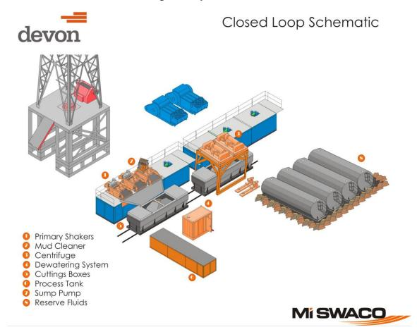
*Centrifuges*: The centrifuges can be one or two in number depending on the well geometry or depth of well. The centrifuges are sized to maintain low gravity solids at 5% or below. They may or may not need a dewatering system to enhance the removal rates. The centrifuges can make a cut point of 8-10 microns depending on bowl speed, feed rate, solids loading and other factors.
