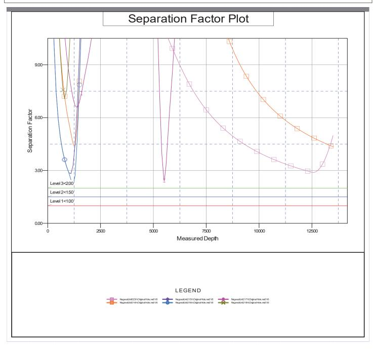
CC - Min centre to center distance or covergent point, SF - min separation factor, ES - min ellipse separation
