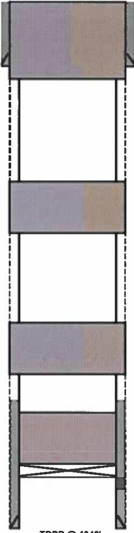
Plug #4: Surface casing Shoe: Squeeze 90 sx Class C cement plug from 380' to 5'.
