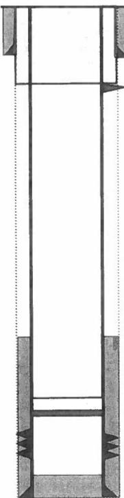
8-5/8", 20# casing set @ 212' Cement w/ 160 sxs, circulated Plug #3: 413'to Surface Class G
