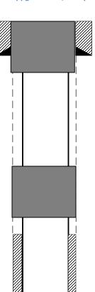
Plug 3 (Surf Csg Shoe) Perf 150' attempt to circ - if circ established, pump total 72 sx cmt, 54 sx cmt annulus to surface, 18 sx cmt inside csg to surf; if no circ, pump 18 sx cmt to surf - top off as necessary
