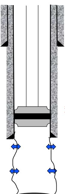
13 3/8" 48# CASING SET @ 321' IN 17 1/2" HOLE CEMENT W/ 500 Sks. TOC @ SURFACE
