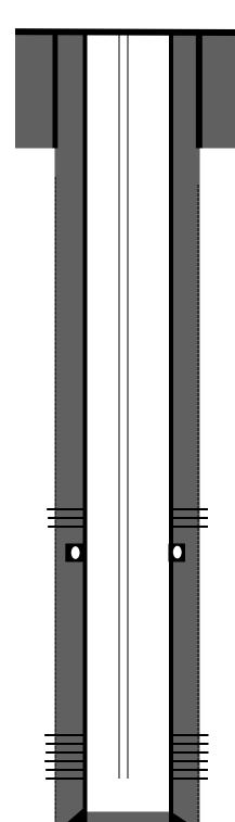
8-5/8" J-55 24# casing @ 293'. Cemented with 175 sks Cement. Circulated to surface
