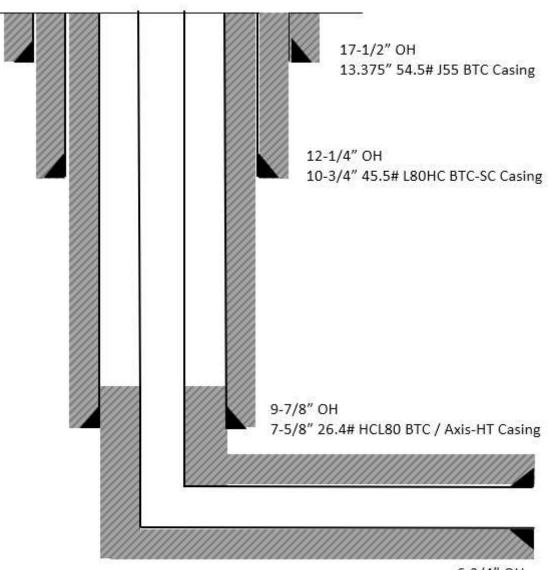
6-3/4" OH 5-1/2" 20# P110 Wedge 461 / Sprint SF / DWC/C-HT-IS Casing TOC @ 500' Above Prev Csg.
