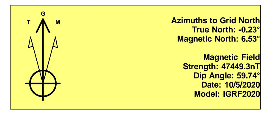
To convert a Magnetic Direction to a Grid Direction, Add 6.53° To convert a Magnetic Direction to a True Direction, Add 6.76° East To convert a True Direction to a Grid Direction, Subtract 0.23°
