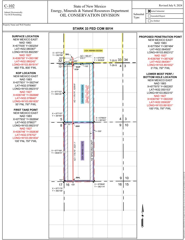
Release Bearings gonglington and distance of grid) shown hereon are based on the New Mexico State Plane Coordinate System, East Zone, NAD 83-2011 (EPOCH 2010) framework, as derived by OPUS Solution. The elevations shown hereon are based on NAVD 88.
