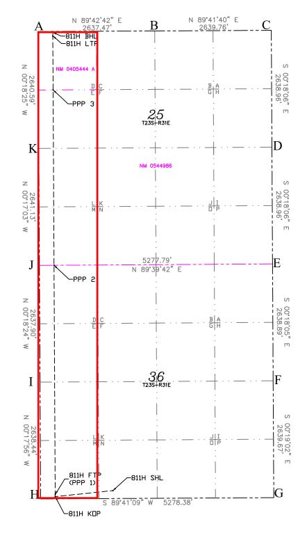
A=N:467082.69 E:724685.21 B=N:467095.96 E:727322.65 C=N:467110.04 E:729962.37 D=N:464471.11 E:729976.26 E=N:461832.19 E:729990.15 F=N:459193.34 E:730004.03 G=N:456553.71 E:730018.64 H=N:456554.76 E:724740.34 I=N:459163.17 E:724726.57 J=N:461801.03 E:724712.45 K=N:464442.13 E:724699.35
