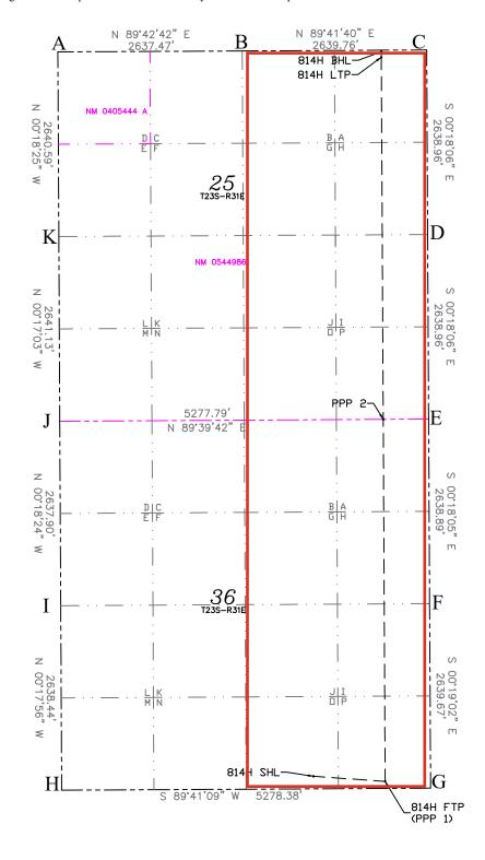
A=N:467082.69 B=N:467095.96 C=N:467110.04 E:724685.21 E:727322.65 E:729962.37 D=N:464471.11 729976.26 E=N:461832.19 F=N:459193.34 729990.15 E:730004.03 G=N:456553.71 E:730018.64 E:724740.34 H=N:456524.76 I=N:459163.17 E:724726.57 E:724712.45 J=N:461801.03 K=N:464442.13 E:724699.35
