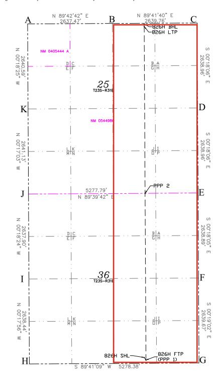
A=N:467082.69 B=N:467095.96 C=N:467110.04 E:724685.21 E:727322.65 E:729962.37 D=N:464471.11 729976.26 E=N:461832.19 F=N:459193.34 729990.15 E:730004.03 G=N:456553.71 E:730018.64 H=N:456524.76 I=N:459163.17 E:724726.57 E:724712.45 J=N:461801.03 K=N:464442.13 E:724699.35
