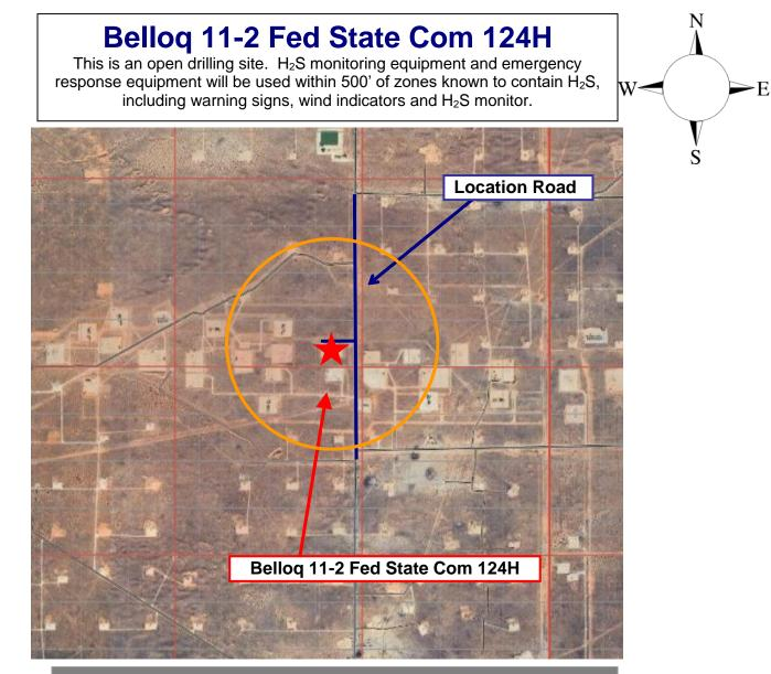
Assumed 100 ppm ROE = 3000' (Radius of Exposure) 100 ppm H2S concentration shall trigger activation of this plan.
