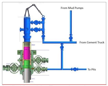
Wellhead diagram during offline cementing operations
