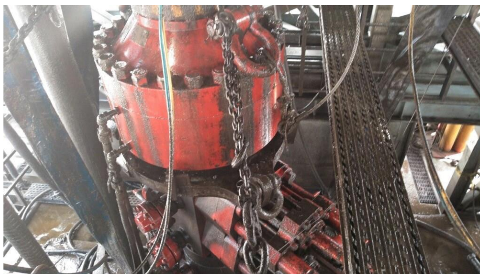
Figure 1: Winch System attached to BOP Stack
