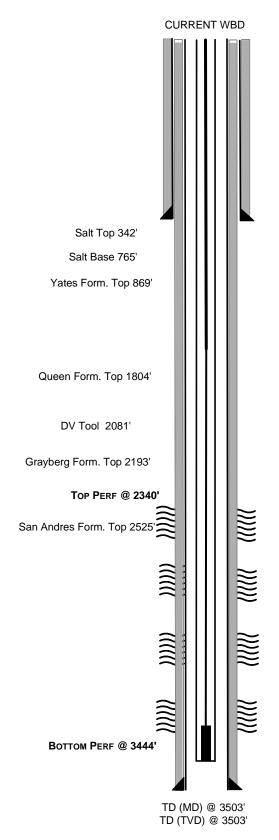
SURFACE 8-5/8" 24# K-55 Csg 0'-325' CMT W/ 350 SXS CLASS C W/2% CACL, ¼#/SX CELLOPHANE, 3#/SX GILSONITE CMT to surface, circulate 140 sxs
