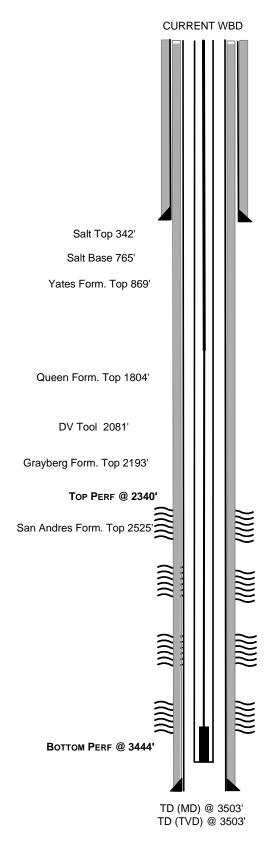
SURFACE 8-5/8" 24# K-55 Csg 0'-325' CMT W/ 350 SXS CLASS C W/2% CACL, ¼#/SX CELLOPHANE, 3#/SX GILSONITE CMT to surface, circulate 140 sxs
