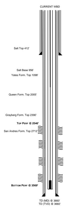
SURFACE 8-5/8" 20# Csg 0'-513' CMT W/ 331 SXS CLASS C W/2% CACL CMT TO SURFACE
