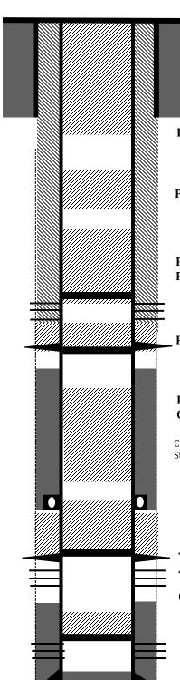
8-5/8" 24# casing @ 228'. Cemented with 135 sks, 159 Cu.ft. Circulated 2 bbls cement to surface
