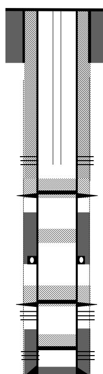
8-5/8" 24# casing @ 228'. Cemented with 135 sks, 159 Cu.ft. Circulated 2 bbls cement to surface
