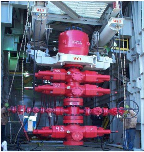
Figure 3. BOP handling system
