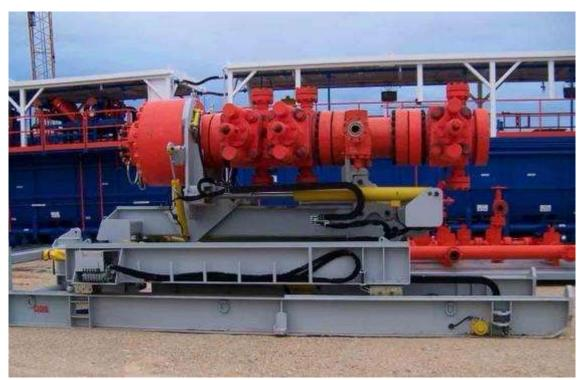
Figure 4. BOP handling system
