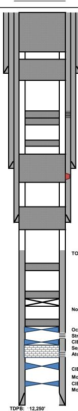
Plug #6: Perf'd @ 2,360'. Sqz'd 630 sxs class C cmt @ 2,360' & circulated to surface.
