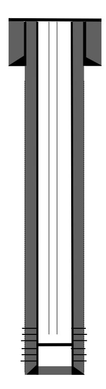
Surface Casing 8-5/8" 20# @177'. Hole size 12  $\frac{1}{4}$ " Cemented w/ 125 sks class B +2%CaCl. Good circ through job, cement circulated.
