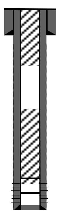
Surface Casing 8-5/8" 20# @177'. Hole size 12 ¼" Cemented w/ 125 sks class B +2%CaCl. Good circ through job, cement circulated.
