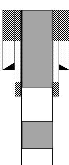
Plug 3 (Surf Shoe) – Perf 188' – attempt to circulate – if circ achieved pump 38 sx cmt for pipe/hole section and 22 sx cmt to surface - if no circ, spot Plug 22 sx cmt 188' to surface Prepared by: BBerry
