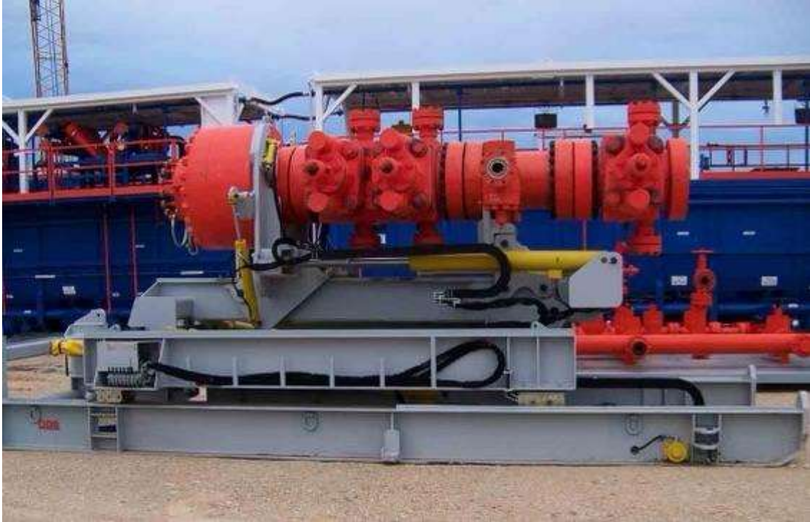
Figure 4. BOP handling system
