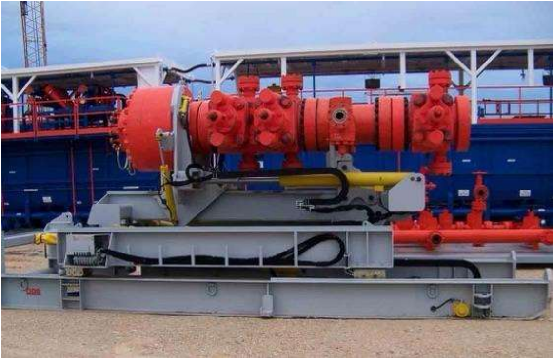
Figure 4. BOP handling system
