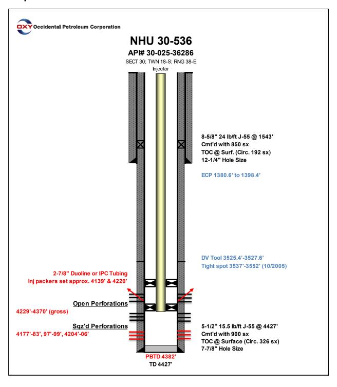
**Objective:** Cement squeeze thief zone (Zn2C) to improve offset production; drill out cement plug to expose Zn3 perfs; add & densify Zn3 perforations.
