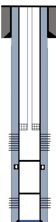
**Surface Casing:** 8-5/8", 24# casing set @ 724' **Cement Job**: 490 sks, Class G cement Circulated cement to surface.
