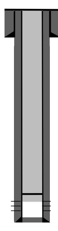
8-5/8" 24# J-55 casing @ 121' Hole size 12-1/4" Cemented w/ 95 sks Type 5 w/ 2% CaCl2 Circ 6 bbls cement to surface
