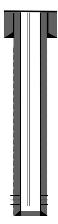
8-5/8" 24# J-55 casing @ 121' Hole size 12-1/4" Cemented w/ 95 sks Type 5 w/ 2% CaCl2 Circ 6 bbls cement to surface
