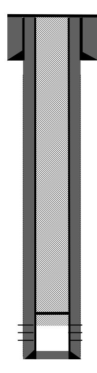
7" 23# casing @ 125'. Spud hole 8 34" Cemented with 55 sks, Class B neat cement (71 cu ft). Circ 2 bbls cement
