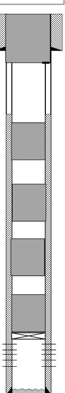
Plug 5 (Surf) Perf 192' – establish circ –pump inside outside plug 95 sx cmt WOC cut off WH install marker – WOC overnight, top off w/cmt to finish Spud Date: 07/09/1982 Completed: 08/23/1982
