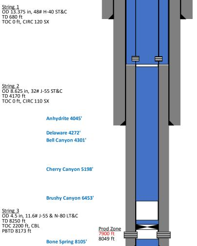
PERF AND CIRC 637 SX CMT FROM 2200' TO **SURFACE. VERIFY CMT TO SURFACE**
