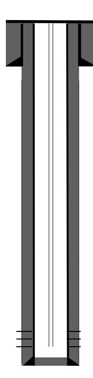
8-5/8" 23#, J-55 casing @ 128': Hole size -12 1/4" Cemented with 85 sks, Class B cement. Circ 4 bbls cement
