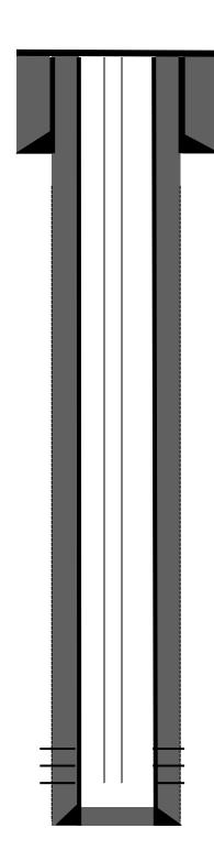
**8-5/8" 24#, J-55 casing @ 136': Hole size -12 ¼"**Cemented with 90 sks, Type III cement, 125 Cu.ft. Circ 6 bbls cement
