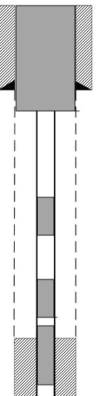
Plug 5 (Surface) – Perf 182' – establish circulation pump 80 sx cement outside plug and 5 sx inside plug cut off WH weld on marker, top off with 10 sx cmt, WOC overnight top off with 1 sack Plug 182-0'
