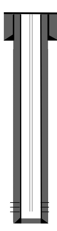
7" 23#, J-55 casing @ 129': Hole size – 8-3/4" Cemented with 60 sks, type 5 cement w/2% CaCl2 w/1/4# celloflake/sx (80 cu ft total slurry) Circ 2 bbls cement
