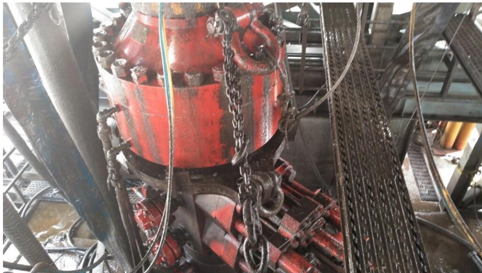
Figure 1: Winch System attached to BOP Stack
