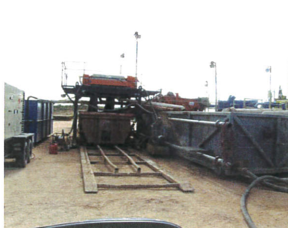
Above: Centrifugal Closed Loop System
