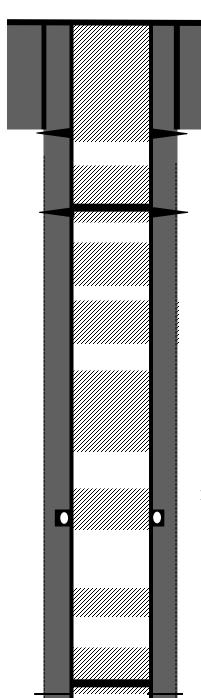
Hole 12 ¼", Casing 8-5/8" 24# @ 259' Cemented w/ 150 sks Class B. Cement circulated.
