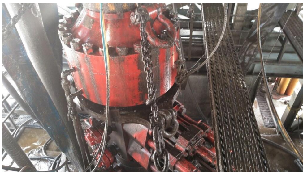
Figure 1: Winch System attached to BOP Stack
